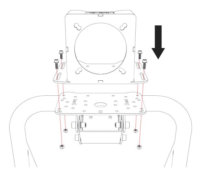
Install the wheel by 4xM8 screws provided. Use 6mm HEX key
