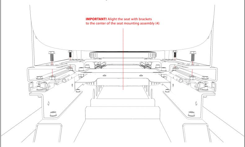
Now adjust the seat position to seat mounting bracket (4) - (height, tilt) and tight the seat using the 6mm HEX Key provided with the assembly.
